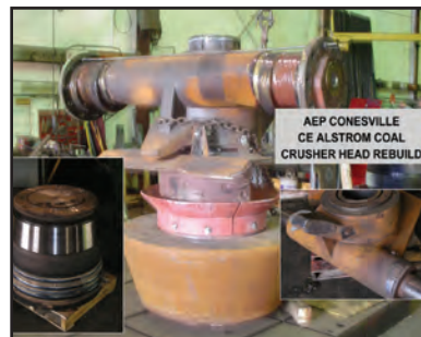
Coal Crusher Rebuild
